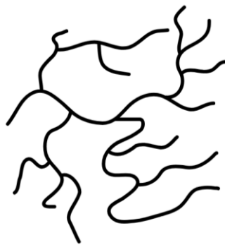
Figure 2.2 Schematic of LDPE branching structure [11].
