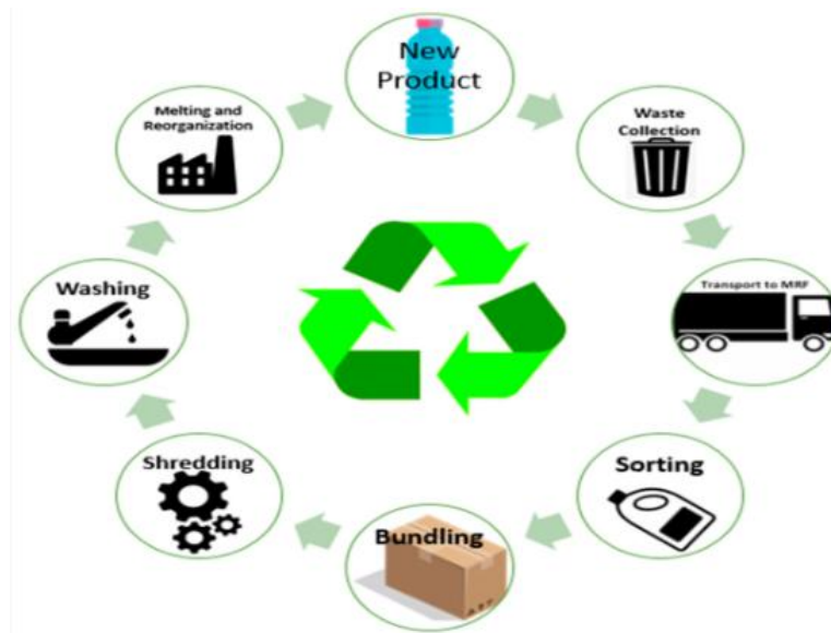
Figure 2.8 Plastic recycling stages [29].
